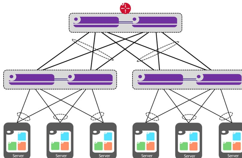
This architecture showcases a Spine and Leaf topology based on a virtual chassis, offering a clear and concise blueprint for seamless integration and automated network management.
