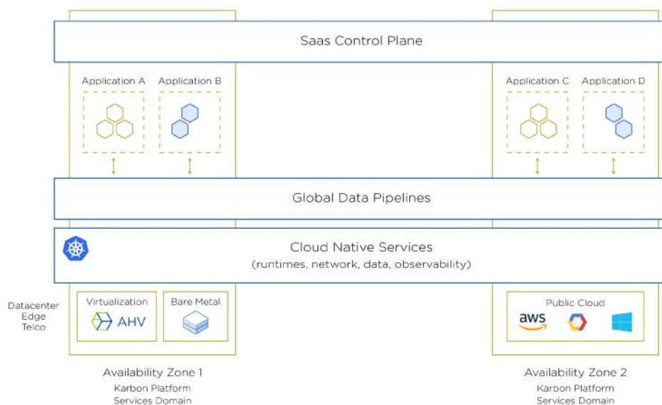
FIGURE 1: Karbon Platform Services Architecture
